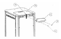
When you take the pellet stove out from its packaging, in the reservoir for pellets you will find the control panel (2) wrapped in a foil and M5 screws (3) mounted on back side of top, which are used for its assembling
