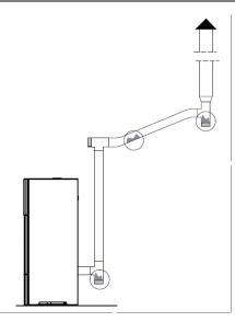
The tar is a liquid which appears when the combustion is poor as a consequence of the low temperature in the pipe. In case of occurrence of tar, it is recommended that the pipe should be isolated well. Deposition of this liquid may cause a fire. So, the exhaust gas system should be checked and cleaned at least once during the heating season.
