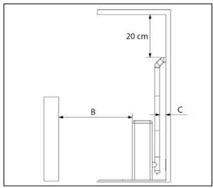
Minimal distance from the flammable materials is 200 mm except dimension explained on picture: A = 200 mm, B = 200 mm, C = 100 mm
