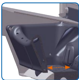
Effective automatic cleaning of the burning chamber.
